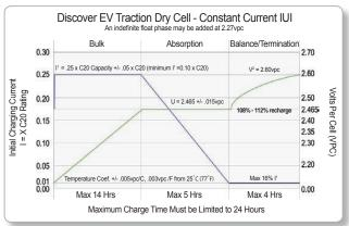
■ NOTE: This algorithm uses a *pulse* termination criterion. As a safety precaution during the *Finish* phase, if the average cell voltage, or volts per cell (vpc), exceeds V2 and the charger output has been on for more than 30 seconds, the output is shut off until the vpc falls to V3. The finish phase then resumes and this "pulsing" continues until the target overcharge (108% - 112%) is reached.
